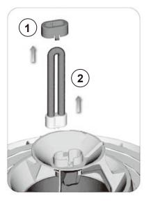
Re-assemble the unit in reverse order. Be careful not to damage the UV-C lamp when putting the filter back in place.
